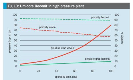
This is true because of the fact that conventional catchment systems can only be used a short time in installations with high primary losses. Since they consist of dense woven gauzes the spaces in-between the meshes quickly accrue and become clogged (Fig. 7). Additionally the pressure drop rises disproportionately which leads to increased stops and downtimes of the reactor. On the other hand, when using a more wide-meshed gauze type, the recovery rate
