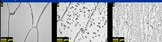
Binary Pt-Ti alloy: Intergranular oxidation only (1); Ternary Pt-Ti-Al alloy: Raising intragranular oxidation with increasing Al concentration (2), (3)
